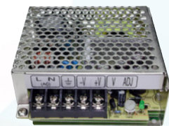
CD-3000+ Power Supply (PS-12V50W-3000)
